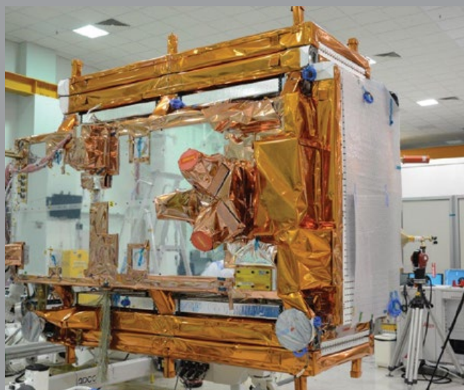
Sentinel-1B after the SAR Antenna integration (Thales Alenia Space)
