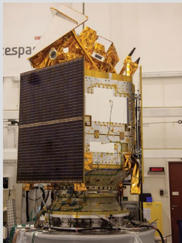
Sentinel-5 Precursor set up for sine vibration test in Intespace (Airbus Defence & Space)
