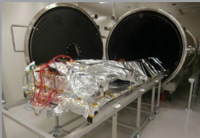
Testing of a large (4 m) sample, in preparation for the Deployable Panel Radiator Qualification testing at EHP, Belgium)
