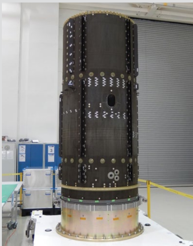
MTG Central Tube STM delivered by RUAG to OHB (OHB)
