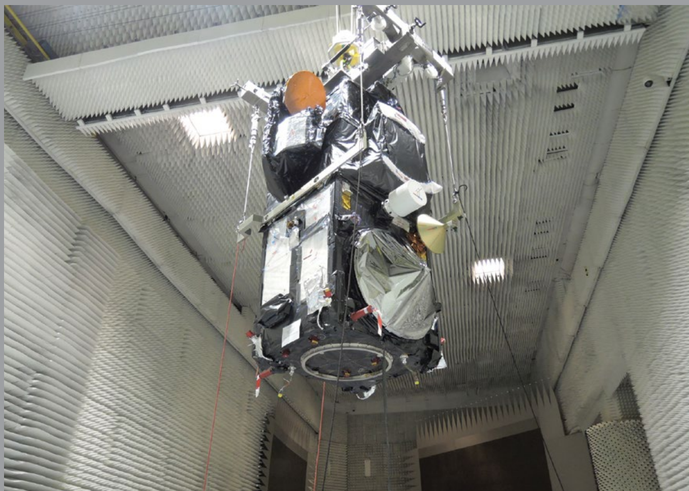
Sentinel-3A in CATR facilities in Cannes during EMC tests (Thales Alenia Space)
